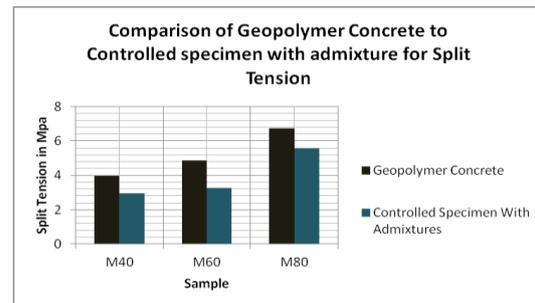
Fig No. 1 Comparison of Geopolymer Concrete to Controlled specimen with admixtures for Split Tension
