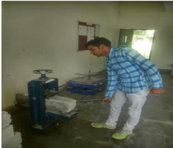
**Fig:7 Flexural Strength Testing.**
