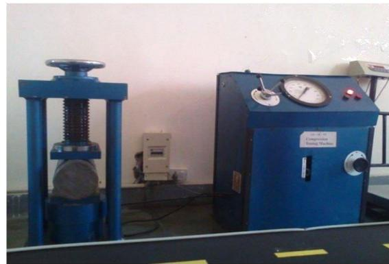
Fig: 5 TEST SET UP FOR SPLIT TENSILE STRENGTH
