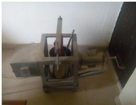
Plate 1: Extracting machine for small-scale production of local pomade from coconut
