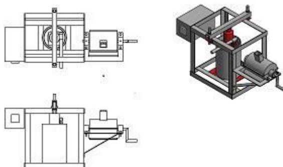
Figure 1: Drawing showing an extracting machine for small-scale production of local pomade from coconut
