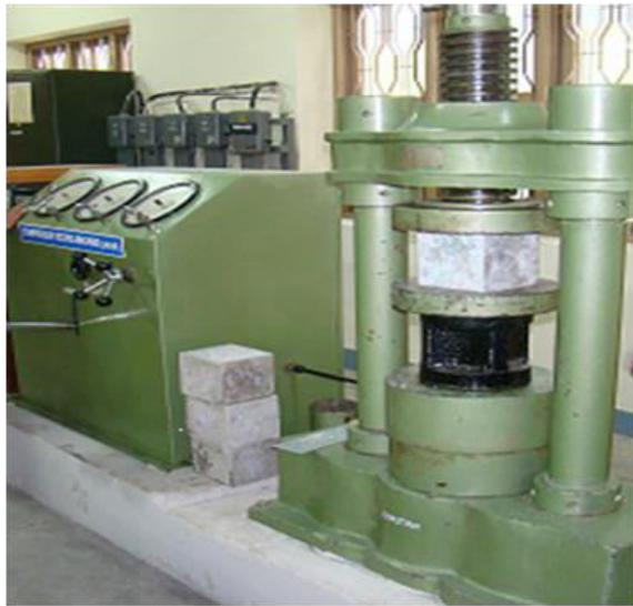
Figure 7. Compression test
