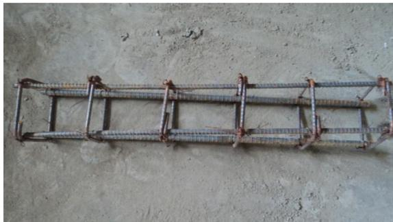
Figure 5. Reinforcement cage.
