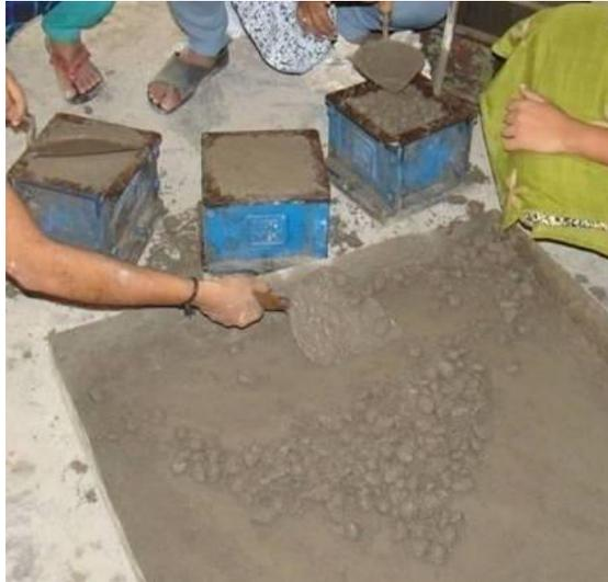
Figure 4. Mixing, Compacting, Finishing of the specimen.
