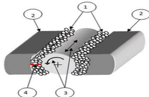
1.Magnetic Abrasives 2.Magnetic Poles 3. Rotation and Vibration of workpiece 4. Working Clearance
