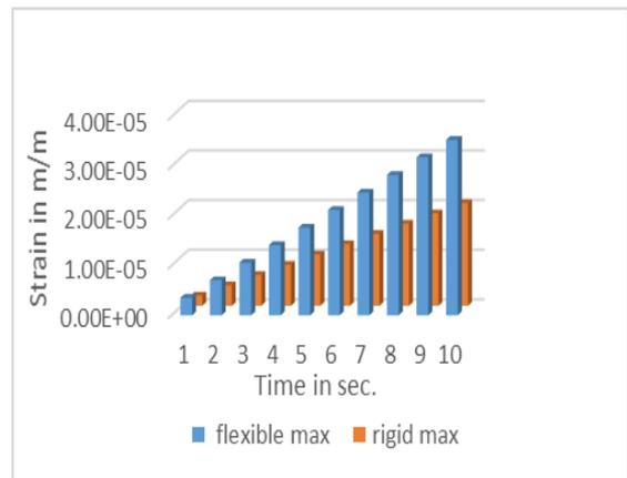
Graph 3 – Strain in flexible and rigid pavement.
