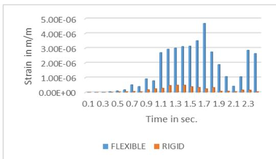
Graph 6 – Strain in flexible and rigid pavement.
