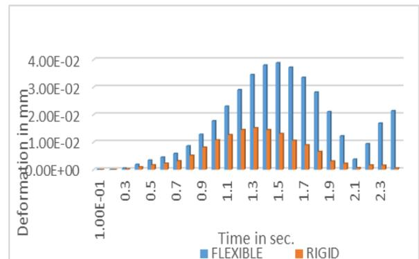
Graph 4 - Deformation of flexible and rigid pavement.
