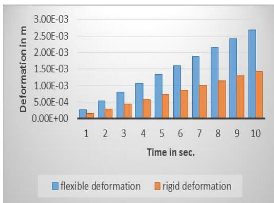
Graph 1 - Deformation of flexible and rigid pavement.
