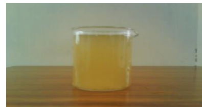
Fig.6. Treated Sago Effluent using Castor Cake
