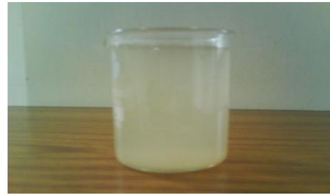
Fig.6. Treated Sago Effluent using Cotton Seed Oil Cake
