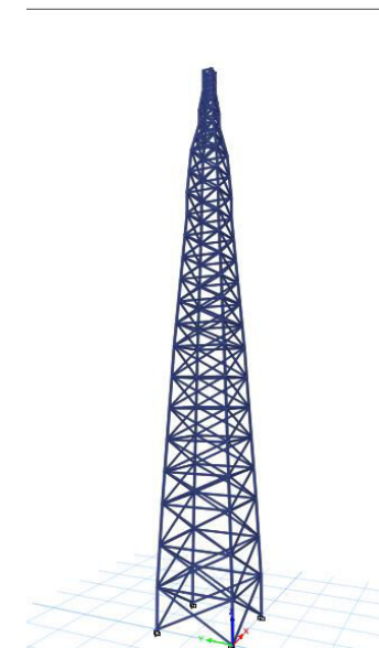
Tower with X Bracing Fig 3
