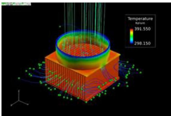
Figure 5. Rectangular heat sink temperature and flow simulation
