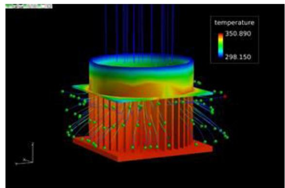
Figure 7. Circular heat sink temperature and flow simulation
