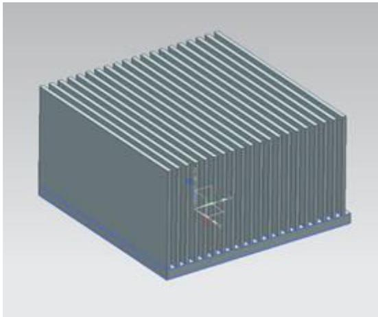
Figure 1. Rectangular heat sink geometry
