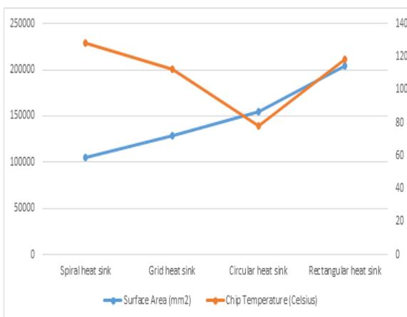
Figure 9: Variation of surface area and chip temperature with heat sink profile
