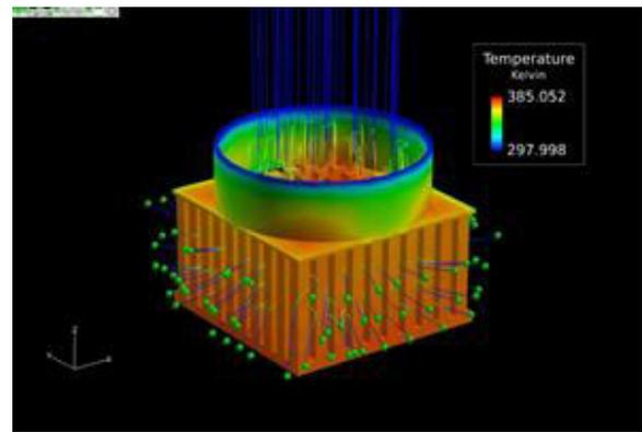
Figure 6. Grid heat sink temperature and flow simulation
