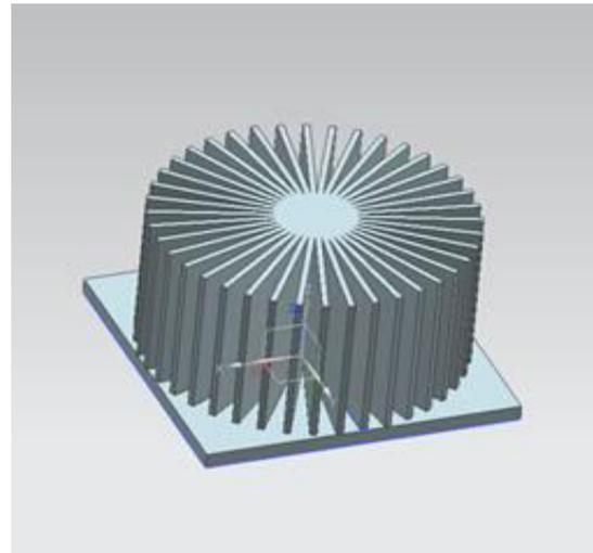
Figure 3. Circular heat sink
