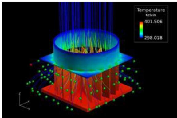
Figure 8. Spiral heat sink temperature and flow simulation
