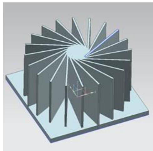
Figure 4. Spiral heat sink
