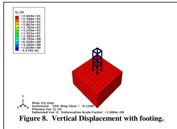
Figure 8. Vertical Displacement with footing.
