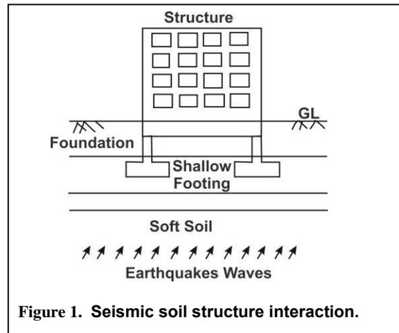
Figure 1. Seismic soil structure interaction.
