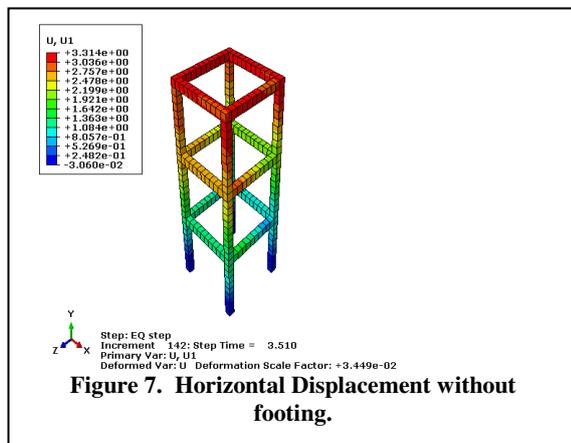
Figure 7. Horizontal Displacement without footing.
