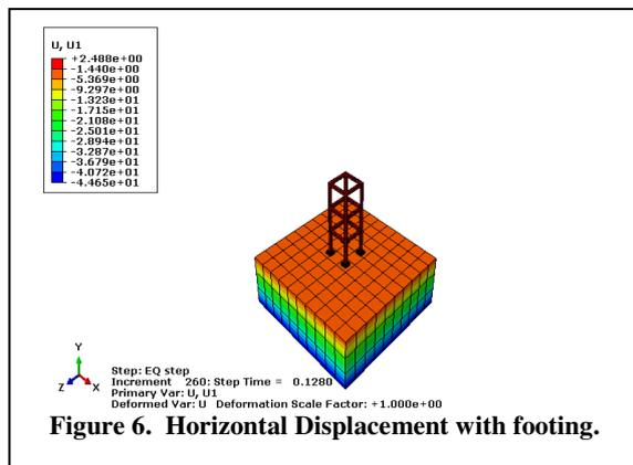
Figure 6. Horizontal Displacement with footing.
