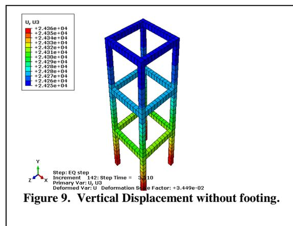
Figure 9. Vertical Displacement without footing.
