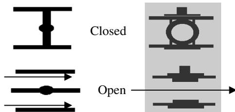
Figure 2 Butterfly Valve      Figure 3 Ball Valve
