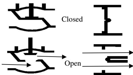
Figure 4 Globe Valve      Figure 5 Check Valve
