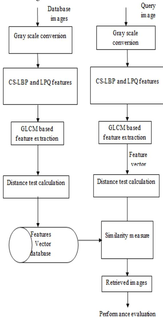
Figure 1: Block Diagram for the System Design
