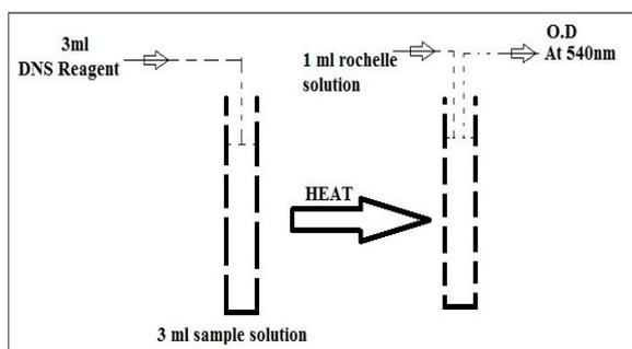
Figure1. Experimental Setup for DNSA method
