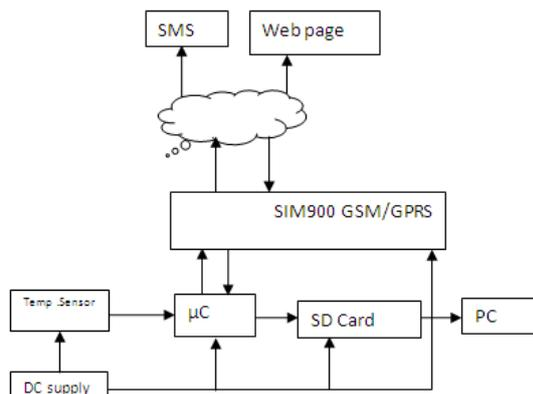
**Fig.5.0: Block diagram of a GSM based temperature remote monitoring system.**
