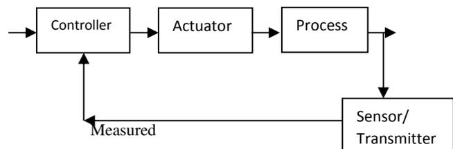
Fig.2.0: Components of a control system
