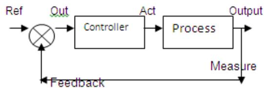
**Fig.4.0: Close-loop Operation**
