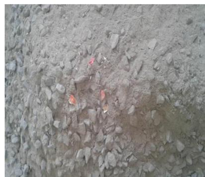
Fig No.2: Steel Waste Fibre added Concrete
