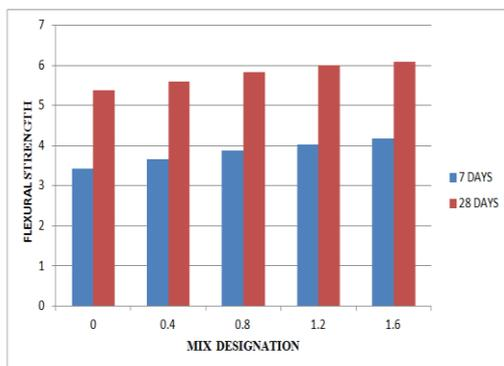
**Fig. No. 5: Graph comparing Flexural Strength for 7 and 28 days**
