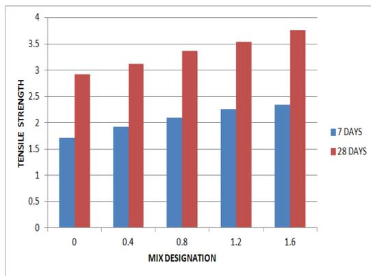
**Fig. No. 4: Graph comparing Split Tensile Strength for 7 and 28 days**
