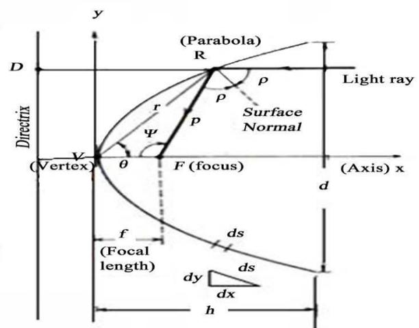
Fig1 Schematic of Parabolic Trough<sup>[1]</sup>
