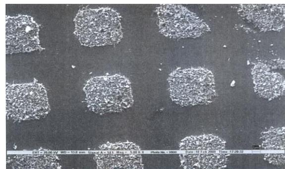
Figure 9. CNTs grown on patterned silicon substrate, each pad (square area of CNTs) is of dimension  $10 \mu\text{m} \times 10 \mu\text{m}$ .
