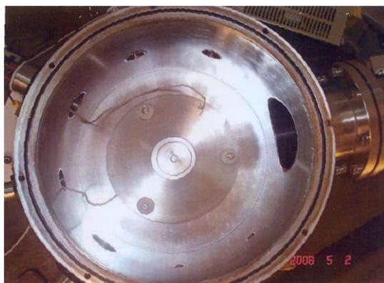
Figure 4: The diode assembly seen from top with the chamber cover open.
