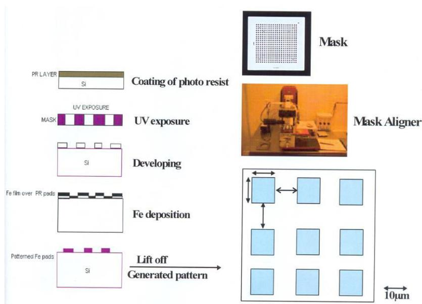
Figure 6. Schematic of photolithography process for generating the Fe deposited patterned structure on silicon wafer
