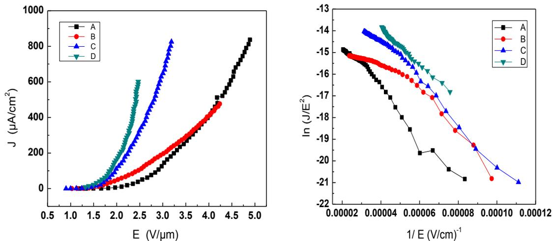
Figure 12. (a) Emission current density versus applied electric field of nanostructured carbon films. (b) Fowler-Nordheim plots of samples A-D.
