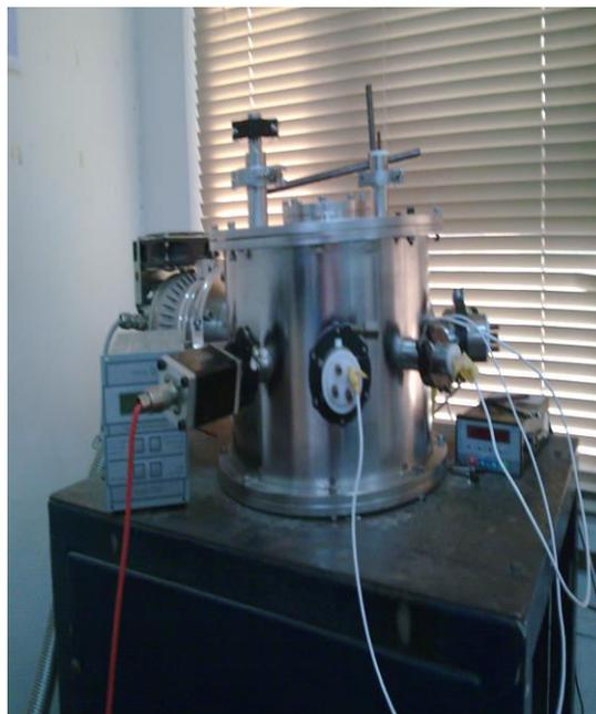
Figure 1. Photograph of the assembled UHV compatible field emission set-up.
