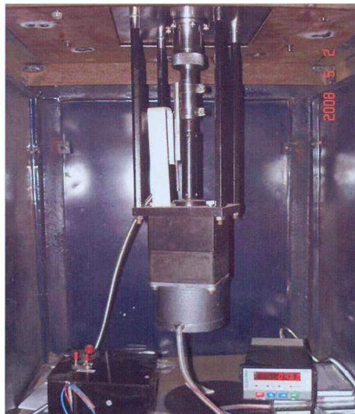
**Figure 3. The digitally controlled cathode movement set up below the chamber.**
