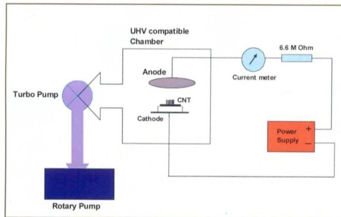
Figure 5. Schematic of the diode type field-emission measurement set-up.
