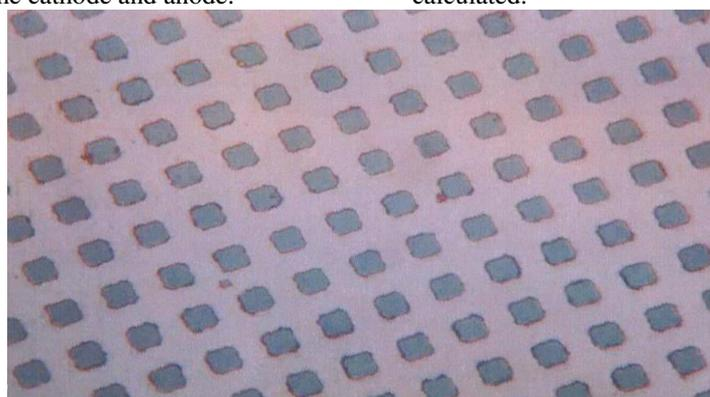
Figure 7. The 10  $\mu\text{m}$  x 10  $\mu\text{m}$  Fe pads seen under an optical microscope.
