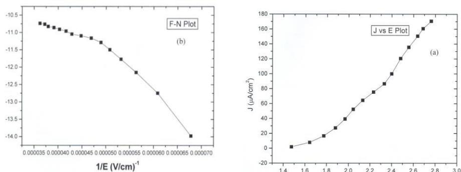
Figure 13 (a) Emission current density versus applied electric field for sample E. (b) The corresponding F-N plot.
