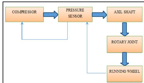
Fig 3 Block diagram of RPMS
