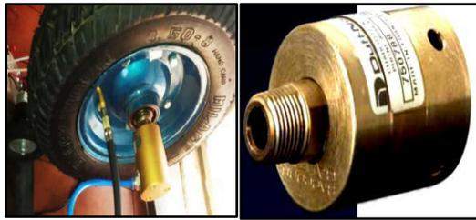
Fig 4 Rotary joints
