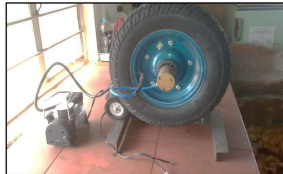
Fig 6 layout and arrangement of running wheel air pressure monitoring system
