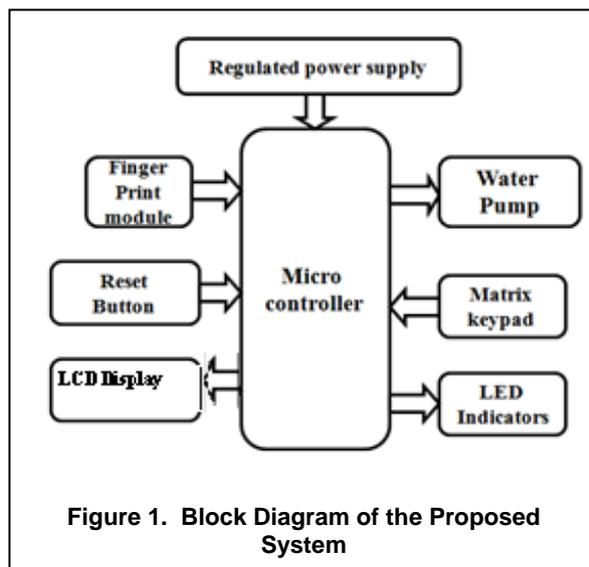
Figure 1. Block Diagram of the Proposed System
