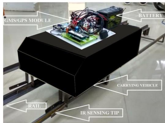
Fig 2: Fabricated Model of Automatic Railway Track Crack Detection System
