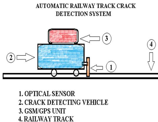
Fig 1: Automatic Railway Track Crack Detection System
