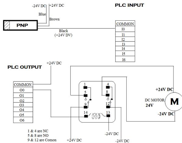
Fig.4. Circuit Connection
