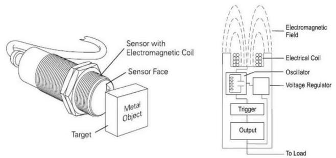
Construction of a inductive proximity sensor
