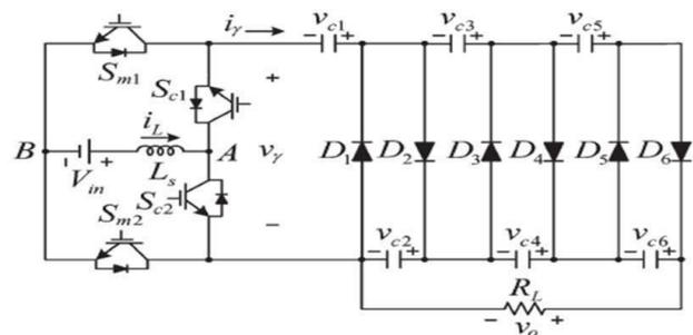
Figure 1 Transformer less Cockcroft-Walton voltage multiplier
