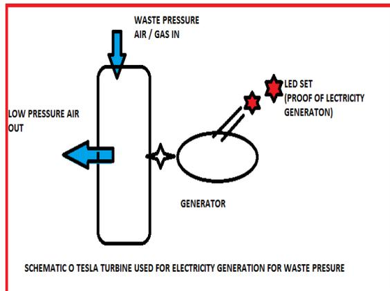
Here the experimental setup will be used to determine and prove the electricity generation from waste pressure. Here input parameter will be Pressure of inlet air and output parameter will be
