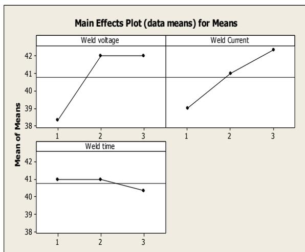
Figure2 Main effect plot for spot welding of stainless steel
