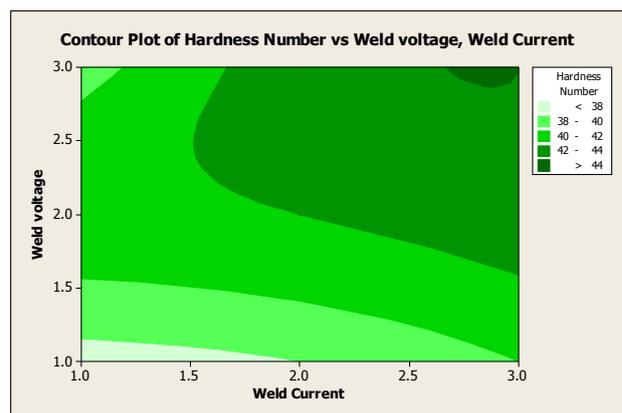
Figure 4 Contour plot of spot welding process parameters
