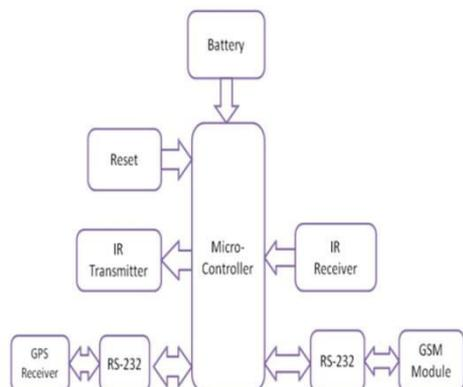
Figure 1: Crack detection using IR.
