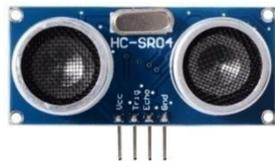
Figure 4: Ultrasonic Sensor
