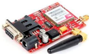
Figure 5: GSM Module
