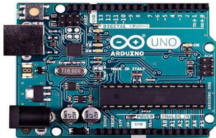
Figure 3: Arduino Uno board.
