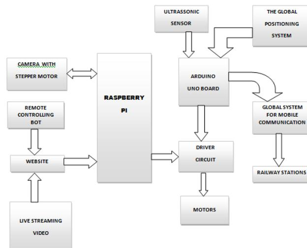
Figure 2: IoT interfaced crack detection system.
