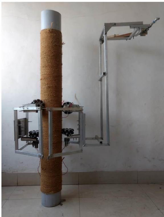
Figure 3. Coconut Demonstration of Electronic Coconut Plucker
