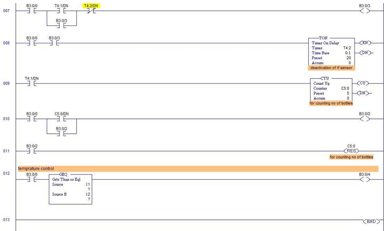
The Ladder Diagram for our bottling system is given like this:
