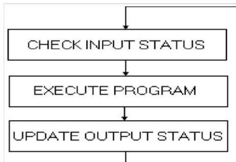
**Check Input Status-** First the PLC takes a look at each input to determine if it is on or off. In other words, is the sensor connected to the first input on? How about the second input? How about the third... It records this data into its memory to be used during the next step.
