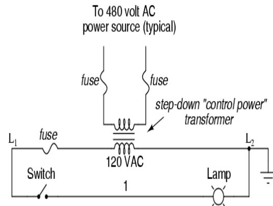
The “L<sub>1</sub>” and “L<sub>2</sub>” designations refer to the two poles of a 120 VAC supply, unless otherwise noted. L<sub>1</sub> is the “hot” conductor, and L<sub>2</sub> is the grounded (“neutral”) conductor. These designations have nothing to do with inductors, just to make things confusing. The actual transformer or generator supplying power to this circuit is omitted for simplicity. In reality, the circuit looks something like this:
