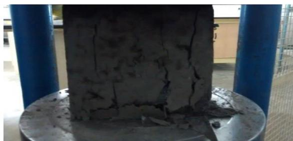
**Figure-5 Compressive strength test SPLIT TENSILE STRENGTH**
