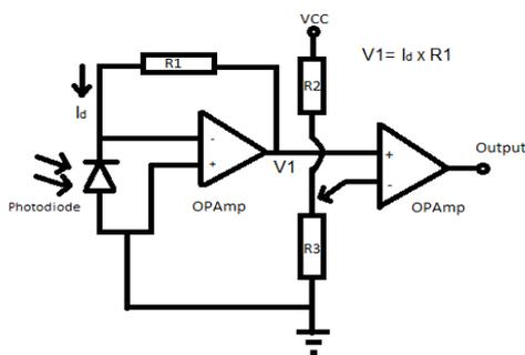
Fig. 4 Circuit diagram for Photo Diode
