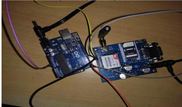
Fig. 7 Arduino UNO board and GSM module(SIM900A)
