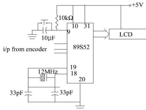
Figure 3. Microcontroller Circuit Diagram
