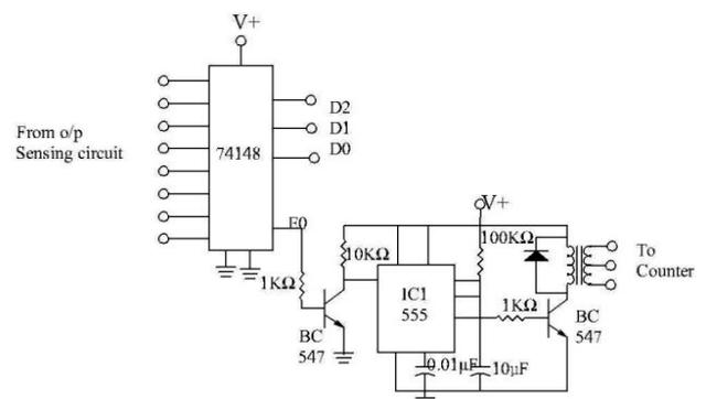
Figure 2. Encoder Circuit Diagram
