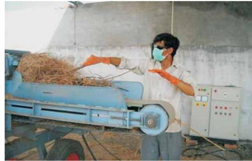
**Figure 4:** Person adding raw material in Biomass briquette machine
