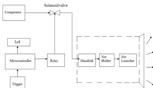
Figure 2: Flow chart for the simple working procedure
