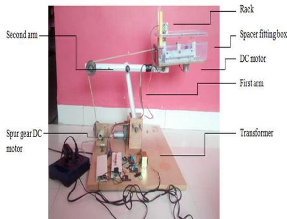
**Figure 3.1: Side View of Project Setup**
