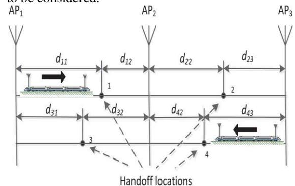
Fig 3. Delay difference between adjacent APs.
