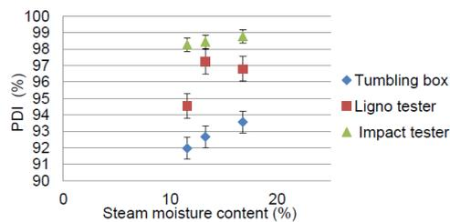
**Figure 3. Pellet durability index (PDI) vs steam moisture content**
