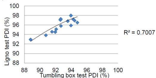
**Figure 6. Correlation between Ligno tester and tumbling box durability tester**
