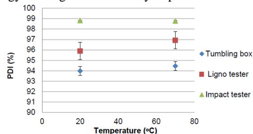
**Figure 5. Pellets durability index (PDI) vs steam conditioning temperature**
