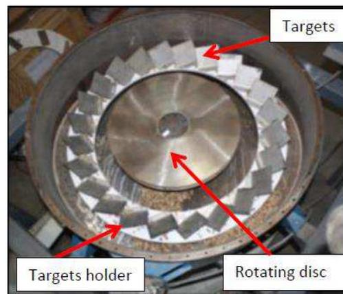
Figure 2. The rotary impact tester after the test (Bradley 1999)
