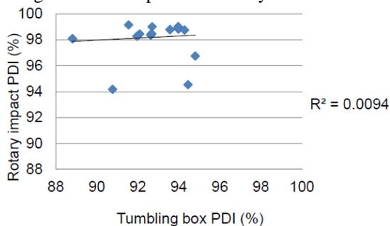
**Figure 8. Correlation between rotary impact vs tumbling box durability tester**
