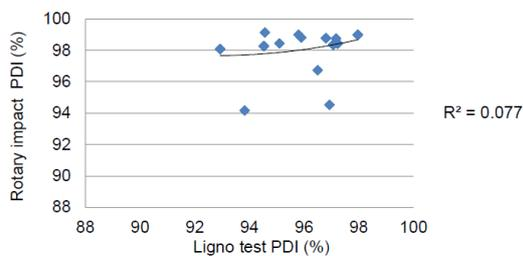
**Figure 7. Correlation between rotary impact vs Ligno tester**
