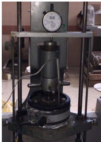
Figure (9). Heater around the Cell.
