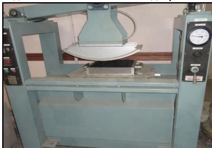
(c) Roller Compaction Machine
