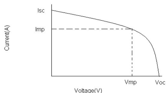
Fig 2 Output Characteristic of PV cell
