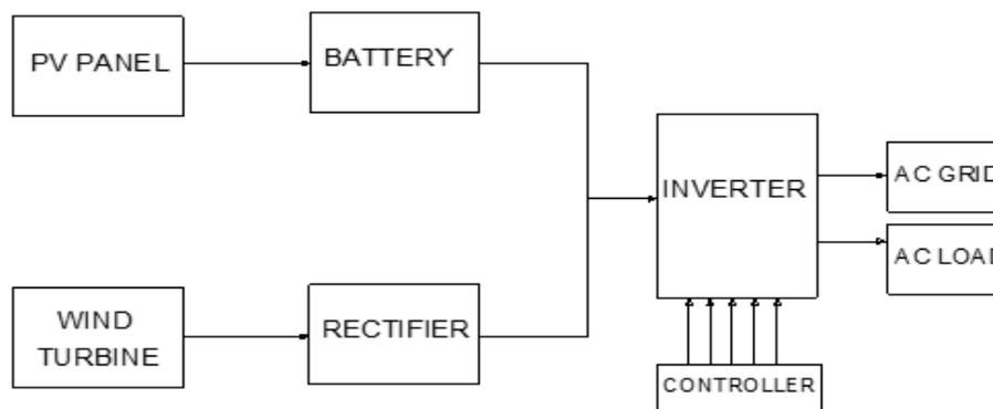
Fig.1 Proposed System Block diagram
