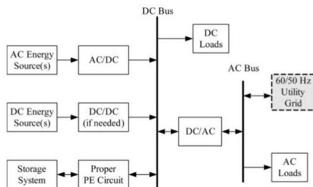
**Fig 3 Schematic diagram of a dc-coupled hybrid energy system**
