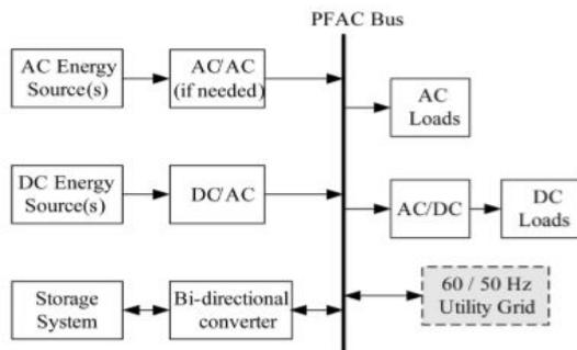
**Fig.4 Schematic of ac-coupled hybrid energy system PFAC**
