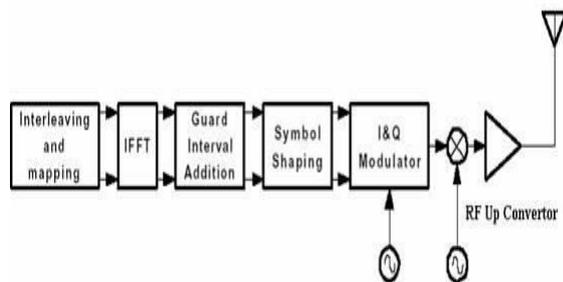
Fig. 1 – Block Diagram of a typical OFDM transmitter.
