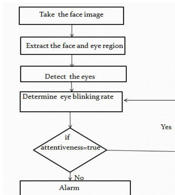
Figure 4. Flowchart of eye detection with Haar classifier
