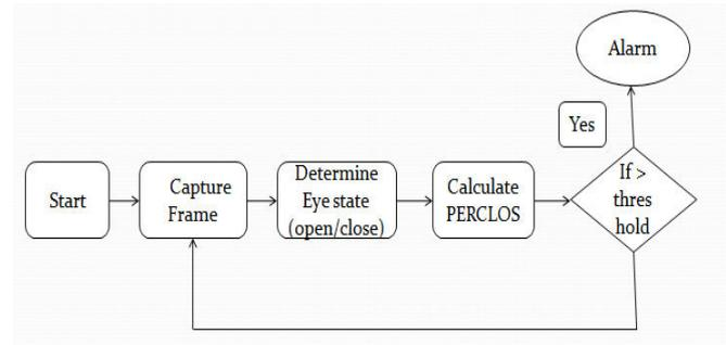
Figure 1. Software Block Diagram
