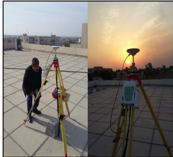
Figure (3): Single receiver set up. (station No.3 on the roof of the chemical industry department building)
