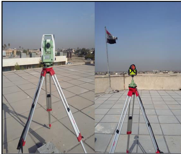
Figure (5): The field observations to create traverse.
