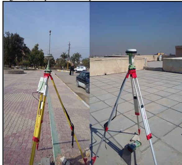
Figure (4): Rapid static of GNSS observation. Base (fixed device on left), Rover (moved device on right).
