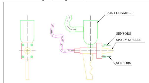
Fig Nozzle design(For Auto wetlayup process)Paint\*Resin
