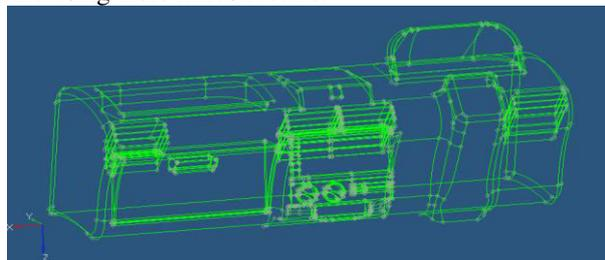
Fig. Wire Frame Model of The Car Dash Board
