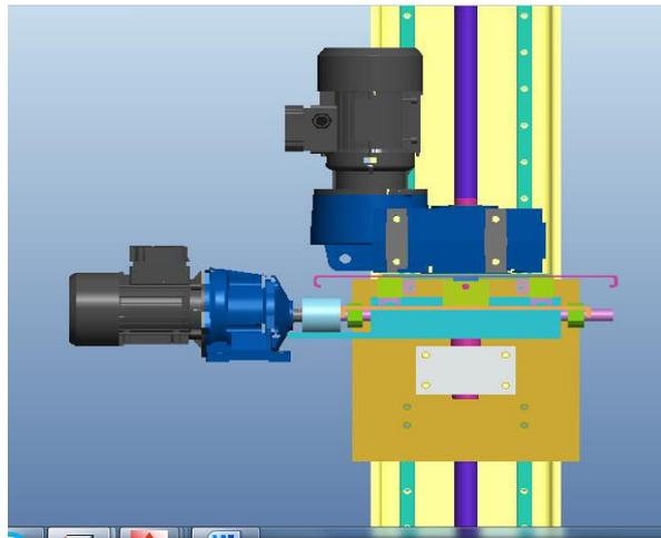
Fig Servo motor setup on the rail
