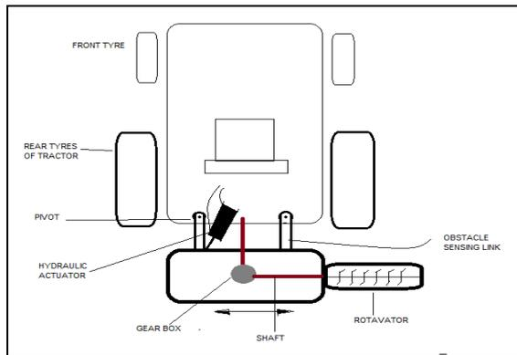
Figure 1 Schematic Representation
