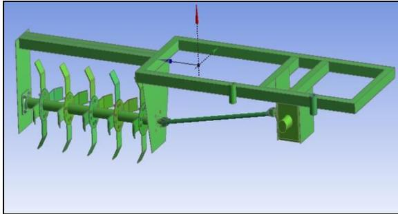
**Figure 5 CAD MODEL OF ASSEMBLY**
