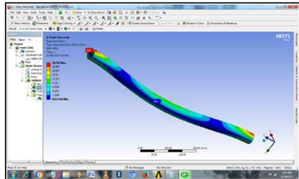
Figure 3 Von Mises Stress ANSYS
