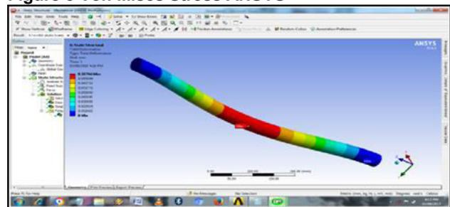
Figure 4 Maximum deformation ANSYS
