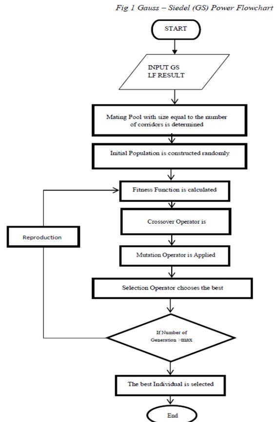
Fig. 2 Genetic Algorithm Flowchart
