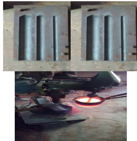
Fig 4.3.3: Die Used For Composites Preparation. Fig 4.3.4: Molten Metal Being Stirred
