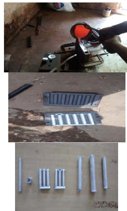
Fig 4.3.5: Molten Metal Poured Into Fig 4.3.6: Casted Composite Metal Preheated Molds
