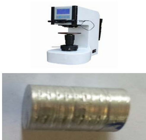
Fig 5.3.1: Brinell Hardness Testing Machine And Specimen After Brinell Hardness Test
