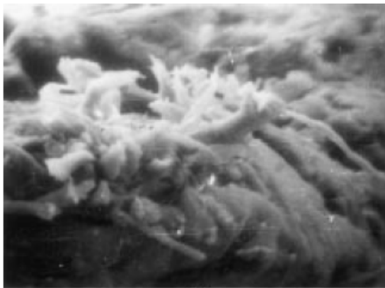
Fig 11.FESEM photographs showing sisal fiber splitting
