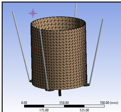
**Figure 7. Meshing of washing machine drum**
