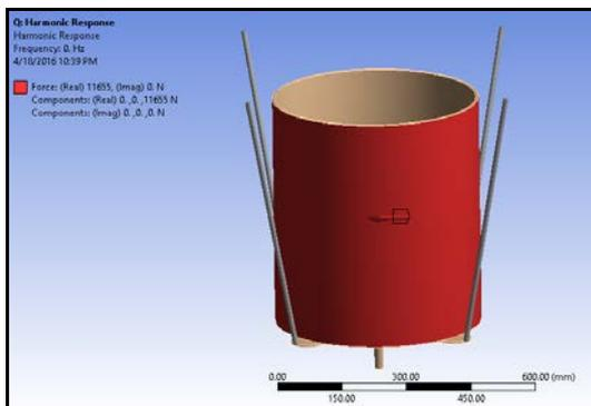
Figure 12. Harmonic Analysis of drum at real force
