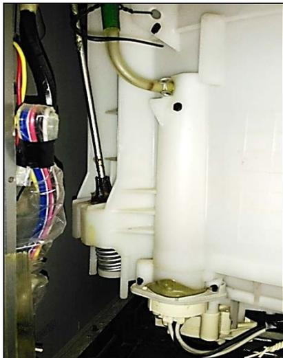
Figure 1 Suspension System of an existing Washing Machine
