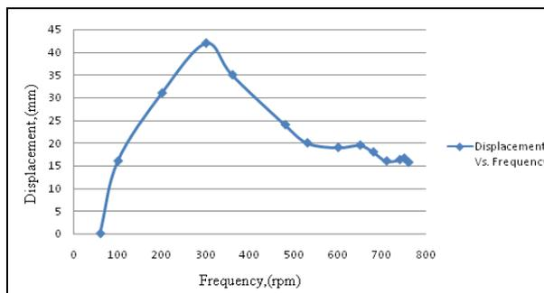
**Figure 21. Frequency Vs Displacement plot for machine with new suspension system**
