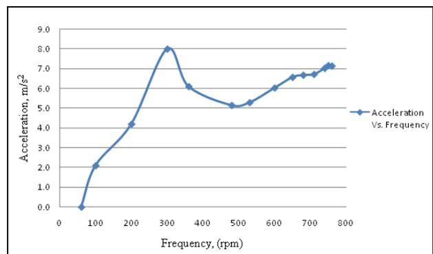
Figure 18. Frequency Vs Acceleration plot for machine with existing suspension system
