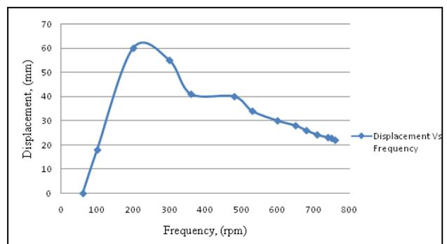
Figure 19. Frequency Vs Displacement plot for machine with existing suspension system
