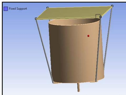
**Figure 8. Boundary condition (Fixed Support)**
