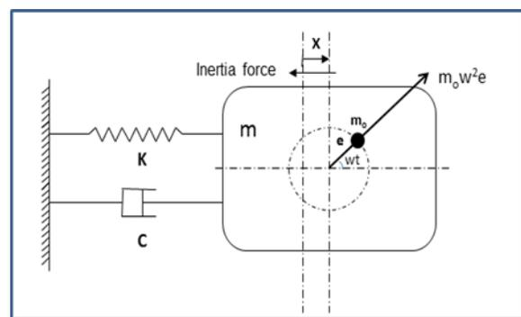
Figure. 3 Free body diagram of washing machine drum
