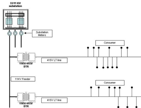
Fig 3. Connection diagram of HVDS
