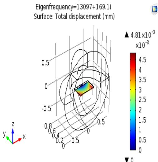
Figure 2 Displacement mode of Al
