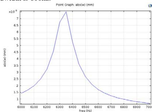
Fig 9 Displacement response of Titanium
