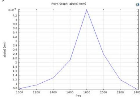
Fig 8 Displacement response of Polyimide
