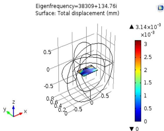
Figure5 Displacement mode of Gold
