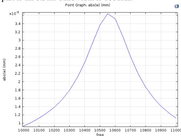
Fig 6 Displacement response of Polysilicon
