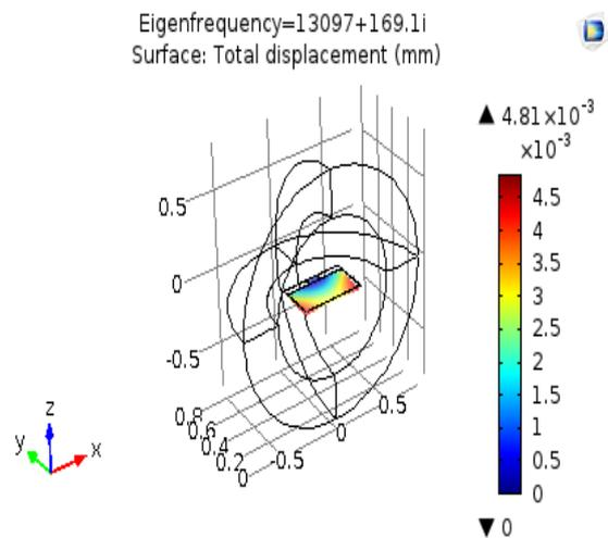
Figure 3 Displacement mode of Polymide
