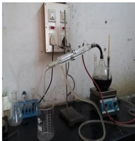
Figure. 7 Methanol Recovery Process
