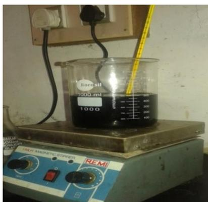
Figure. 9 Drying of Biodiesel
