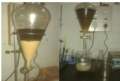
Figure.8 Water Washing process of Biodiesel
