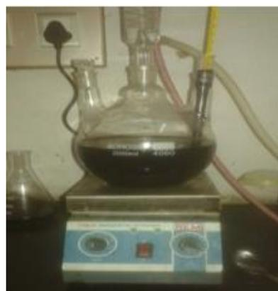
Figure. 4 Three Neck Reactor with Magnetic Stirrer with Hot Plate
